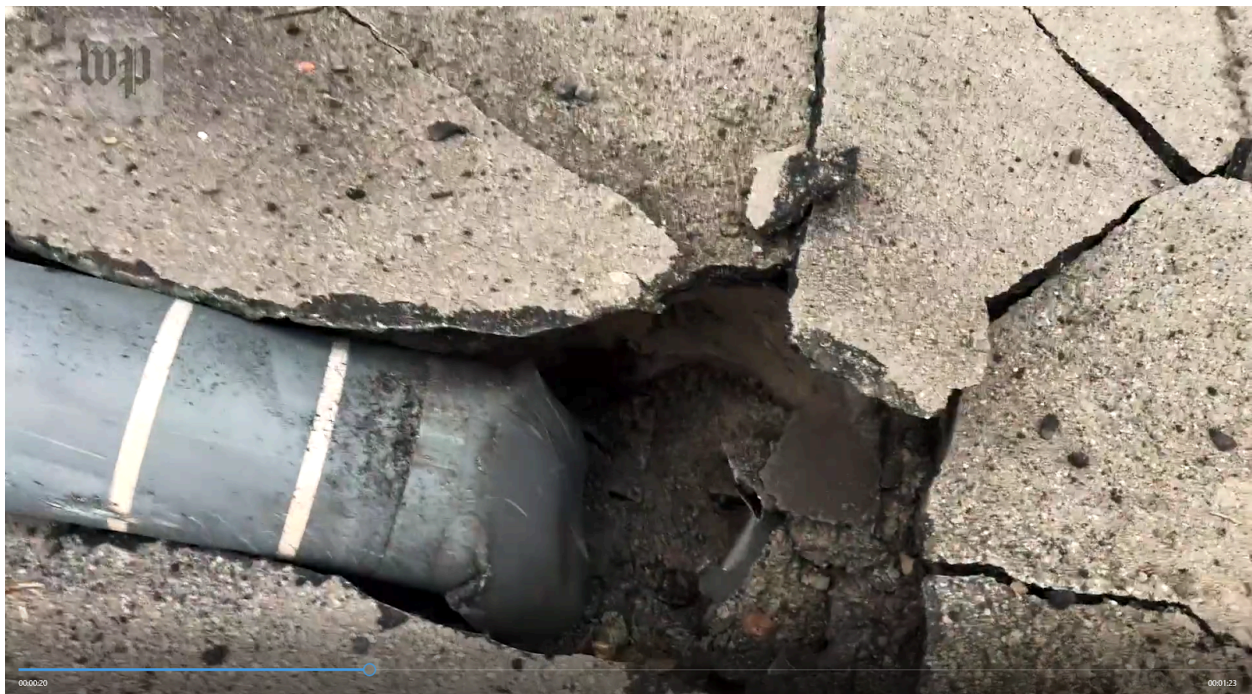
Still from S8V1 clearly shows how the rocket motor has buckled.
