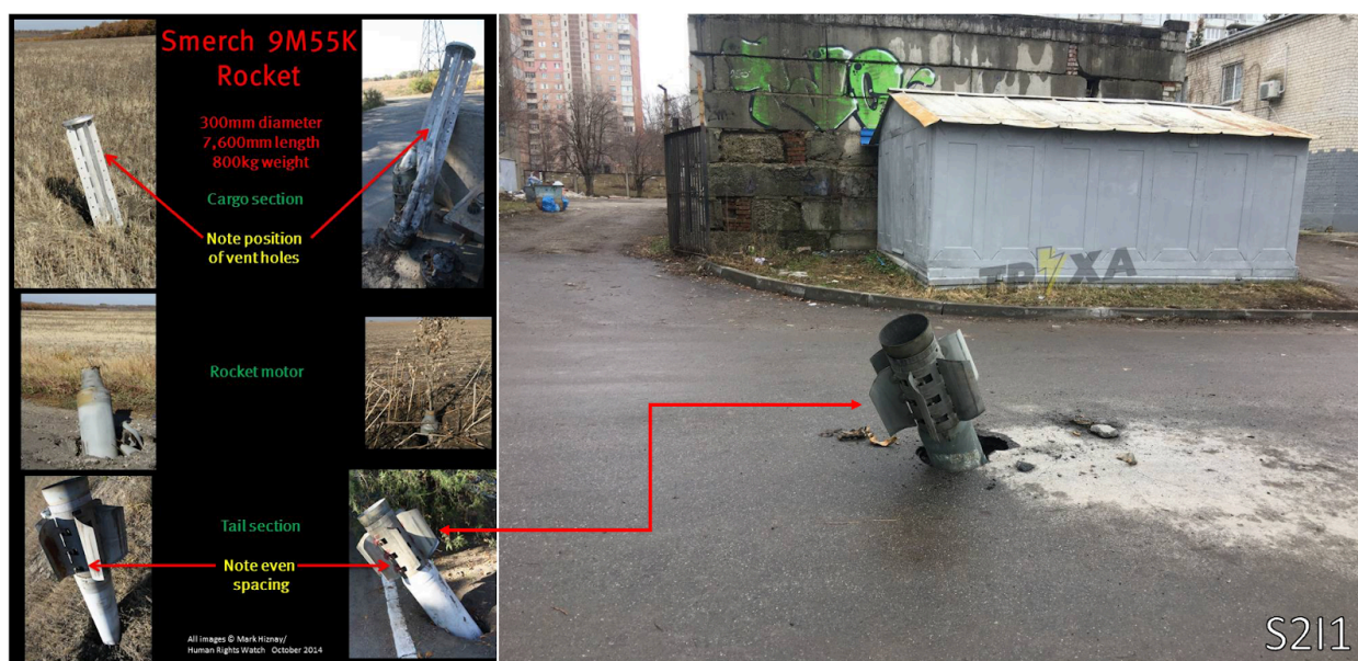
Left: Recognition card created by Human Rights Watch associate director of the Arms Division, Mark Hiznay 20 . Right: S2I1 depicting Fragment 3. Note the even spacing between the three hinges of the tail section.
