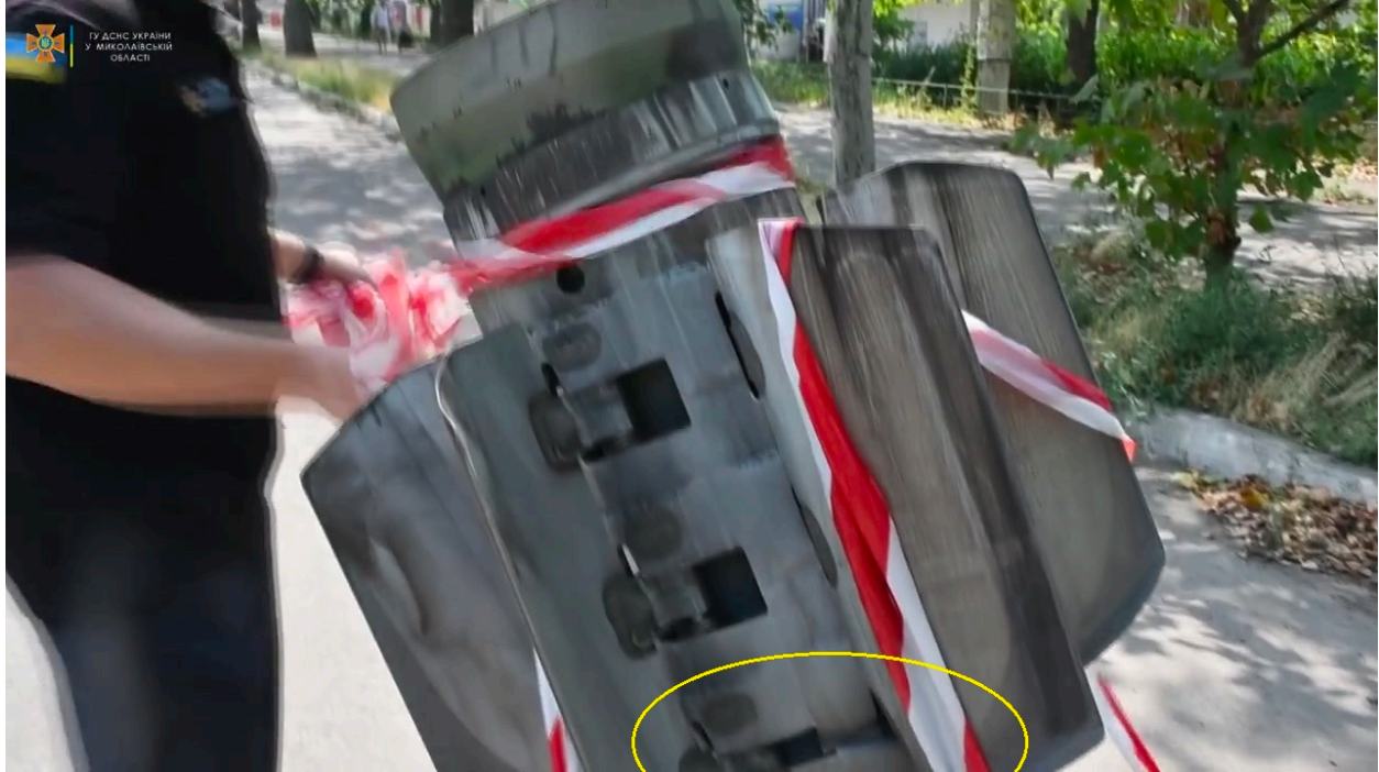
Example of a buckled collar on a 9M55K identified in a Facebook post 16 by the Mykoliav State Emergency Service.
