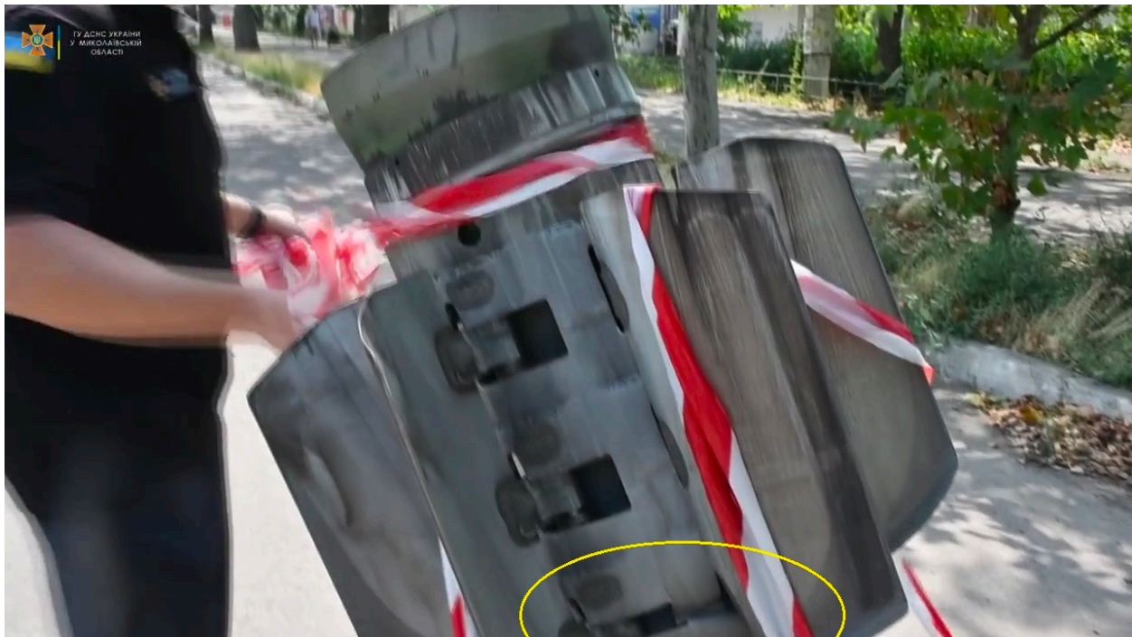
Still frame from the video 12 depicting a 9M55K rocket motor being collected after the impact. Note how the tail section has been forced down, bending the hinge hole.
