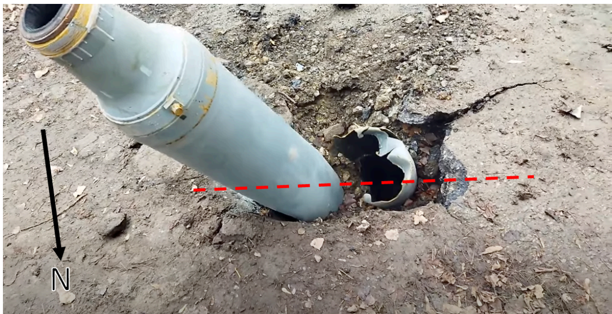
Still from S2V1. Note the linear nature of the damage caused to the asphalt indicated by the red line, as well as the shearing of the rocket motor.
