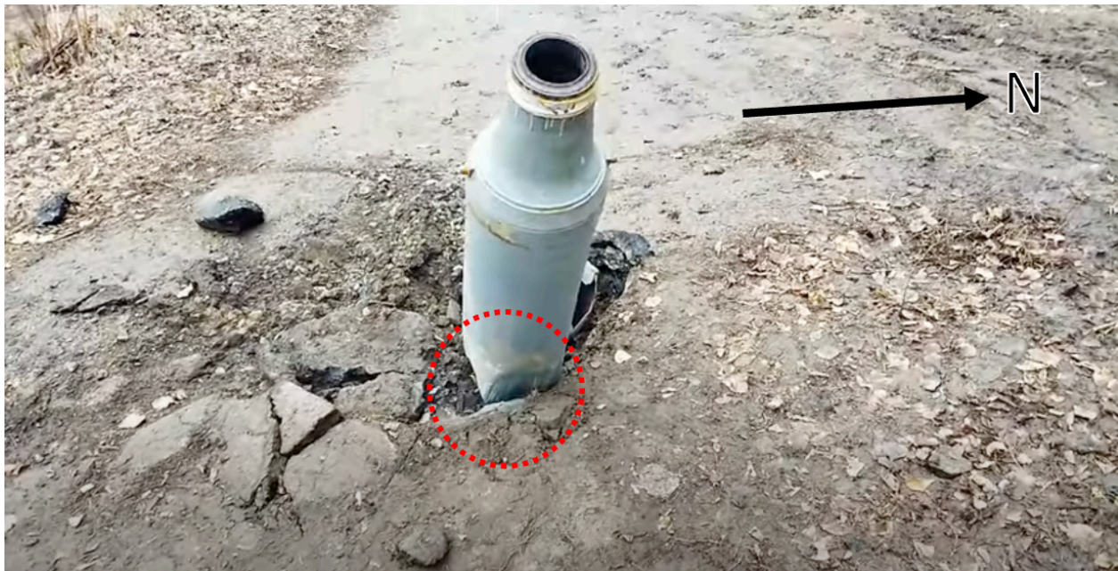
Still from S2V1. Note the damage caused to the eastern side of the rocket motor highlighted by the red circle.
