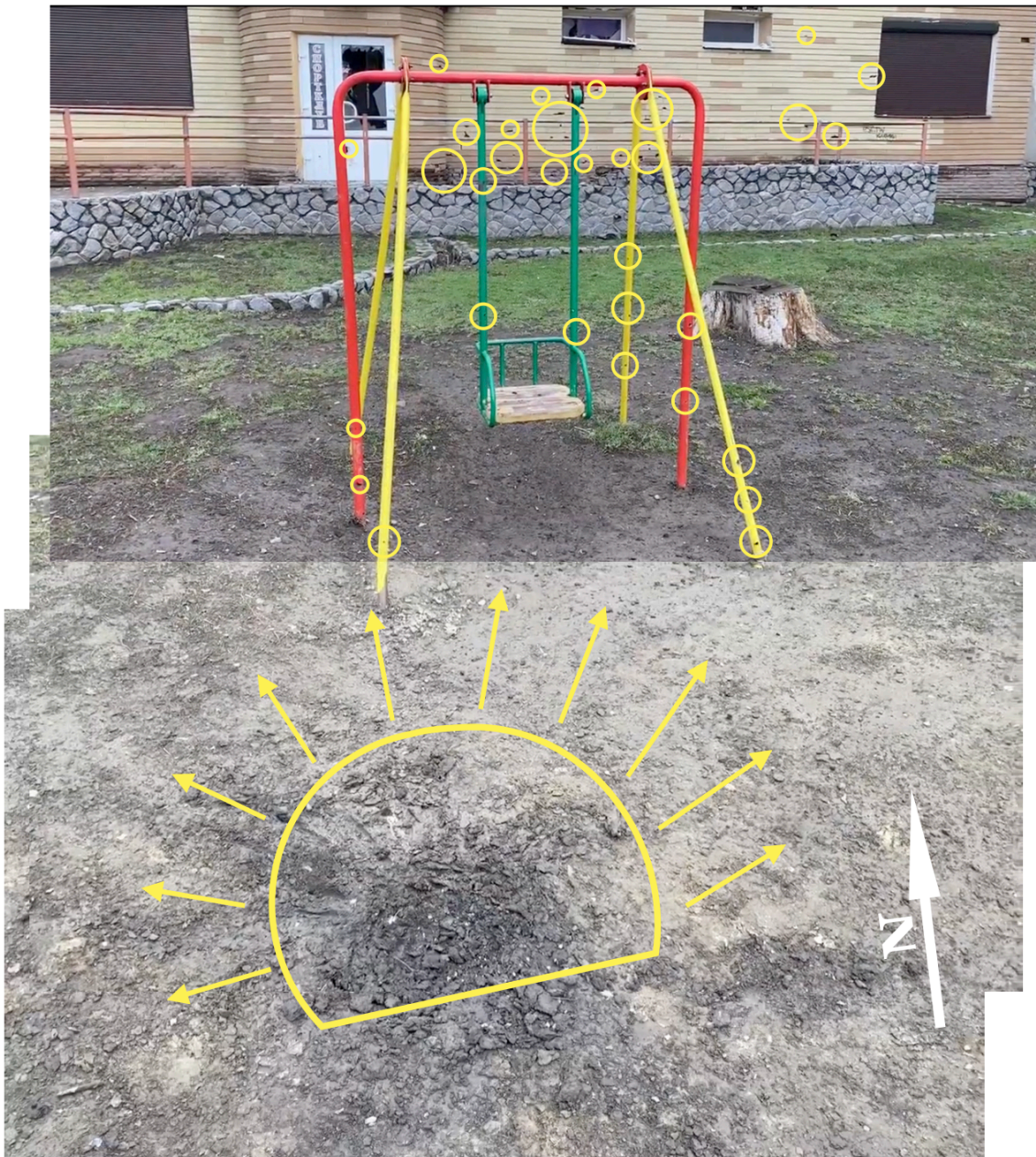
The size and amount of marks, and the direction of fragmentation of 9N235 submunition correspond to marks and holes on the children's slide visible at the CIVO761A scene (S13V1).
