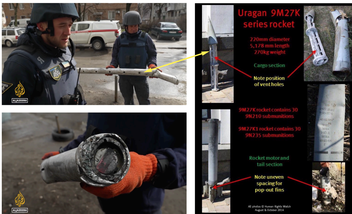
Visual comparison of the pipe found at the location of CIVO761J and depicted on S9V1 (Left) with the reference imagery depicting cargo sections of an Uragan 9M27K clutter munition rocket (Credit: Mark Hiznay/Human Rights Watch).
