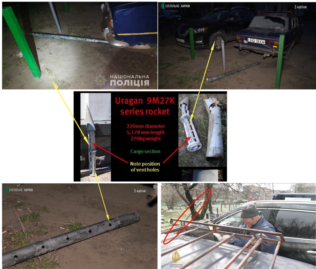
A visual comparison of the pipe depicted at the location of CIV0761I on S12I4 (Top Left); S7V1 (Bottom Left and Top Right); and S9V1 (Bottom Right) with the reference imagery (Center) of cargo sections of a Uragan 9M27K cluster munition rocket (Credit: Human Rights Watch).
