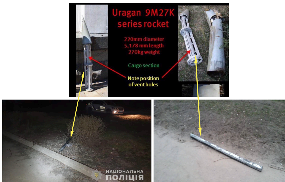
Comparison of metal pipes with vent holes depicted on S12I6 (Bottom Left) and S3I1 (Bottom Right) with the reference imagery (Top) of an Uragan 9M27K rocket (Credit: Human Rights Watch).
