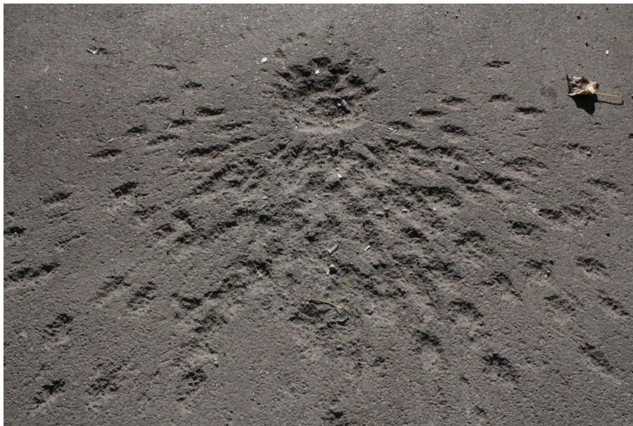
Fragmentation pattern on a hard surface caused by a 9N210 submunition impact outside the ICRC office on Universitetskaya Street, Donetsk, October 2014 (Credit: Harriet Salem 63 ).
